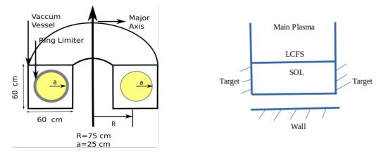
[Left hand side Fig.1 is the Schematic of Aditya ring limiter tokamak, Right hand side Fig.2 is the simple 1D slab model of SOL region]
